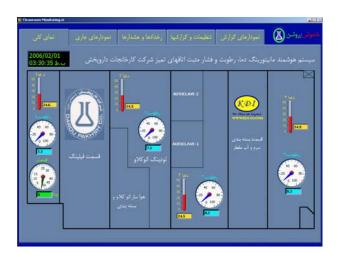
The system monitors temperature, humidity, differential pressure, particle number and airflow speed of the cleanroom.
