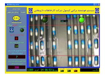
The system inspects blister packages to detect missing or broken contents, wrong colored/shaped contents in the cells.
