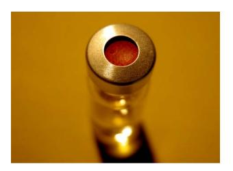
Pharmaceutical caps are inspected for defects in the rubber insert and in the aluminum cap. As an add-on the system can inspect the holes in the rubber band from which the rubber insert is punched.
